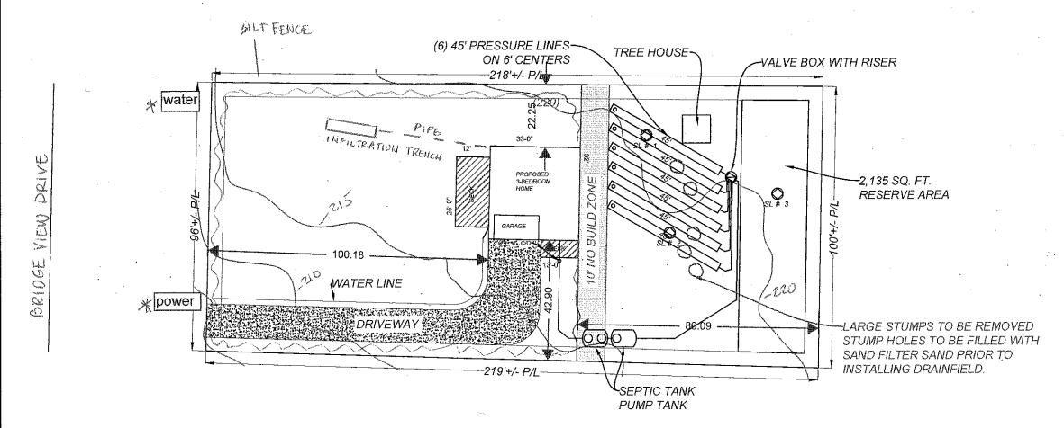
Do not Damage Or Disturb Soils When Clearing Drainfield Area
