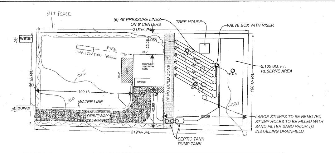
Do not Damage Or Disturb Soils When Clearing Drainfield Area
