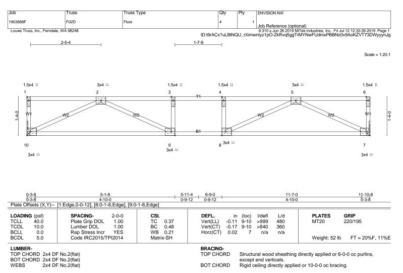
REACTIONS. (lb/size) 7=646/Mechanical, 10=646/Mechanical
