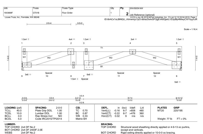
**REACTIONS.** (lb/size) 6=2182/Mechanical, 9=2125/Mechanical
