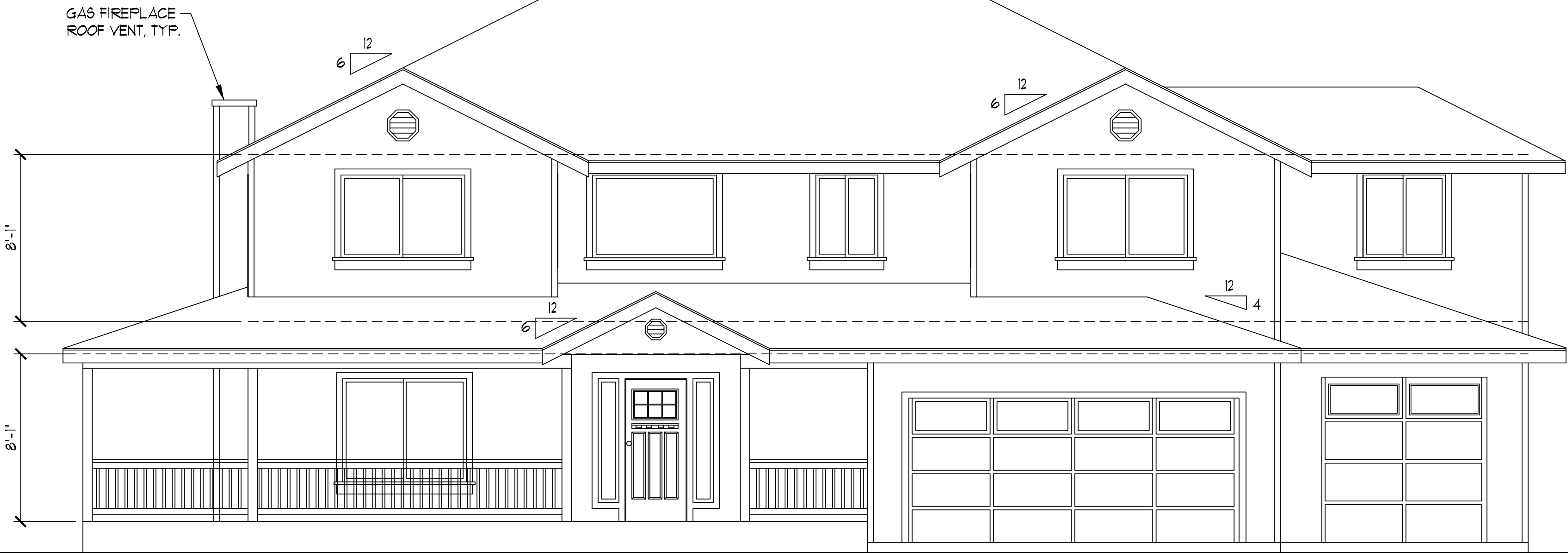
FRONT ELEVATION SCALE : 1/4" = 1'
